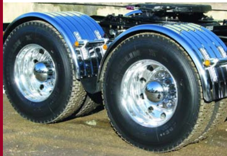
Michelin 11R22.5 are fitted to drive and trailer axles.
