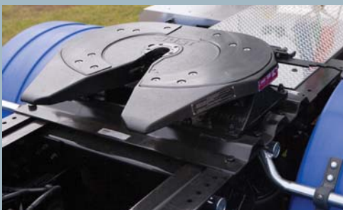
Transmissions are manual shifting with Autoshifts preferred for the future. Jost 5th wheels are grease-free with low friction inserts.
